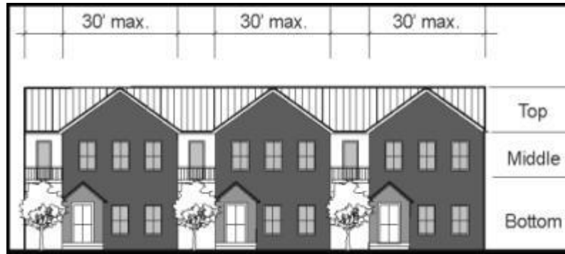
Figure 3 – Note the repeating distinctive window patterns and the articulation of the building's top, middle and bottom.
