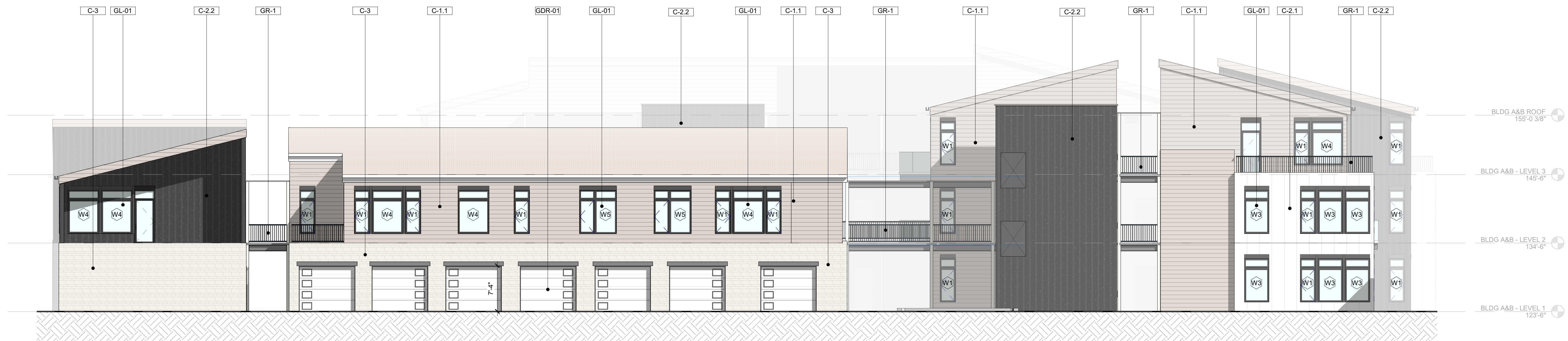
2 BUILDING A - SOUTH ELEVATION 1/8" = 1'-0"
