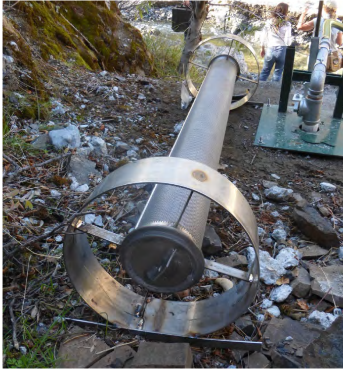
Figure 8-10 Typical end-of-pipe screen equipped with “wagon wheels” to elevate the screen off the stream bottom
